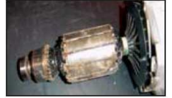
Armature burnt out (overloaded)
