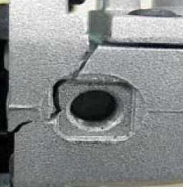
Fractured housing caused by drop
